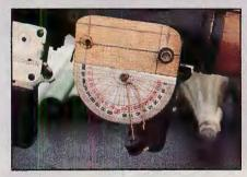
Improvised clinometer attached to left side of RPG-7V by FMLN for the slant range computation required to effectively employ 81mm mortar bomb mated to PG-7 rocket mater.
